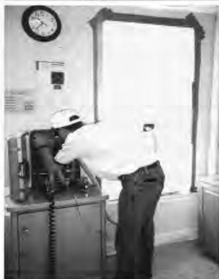
Technician monitors equipment for a field test of a newly installed storm window to make sure it meets the requirements of air leakage no greater than 0.5 CFM per lineal foot of sash crack.
